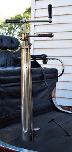
Fig 3: Vertical steering column with rear-mounted exhaust valve control and the horizontal lever that enables both gear changing and rear wheel braking.
