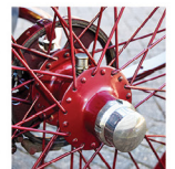
Fig 7: Rear wheel plain bearing hub with the pronounced central bulge and transfer grease.
